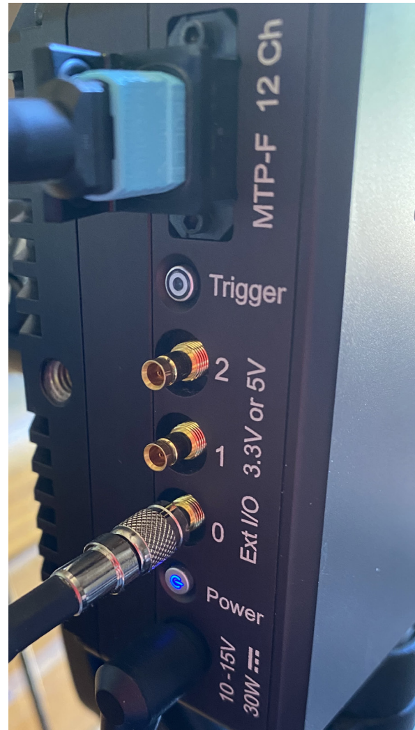
Figure 2-9: External I/O Connections
