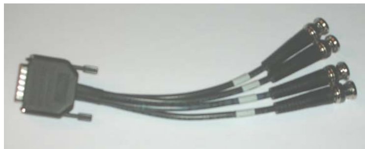
Figure 3-2: DB-15 Multiple I/O Camera Interface Cable
