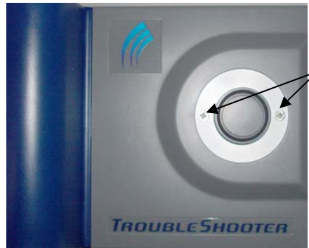
Figure 2-3: Back-Focus Ring Retaining Screws
