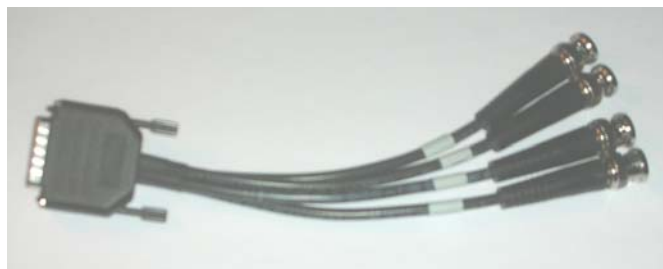
Figure 1-4: DB-15 Multiple I/O Camera Interface Cable
